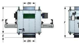
The Dosing device is available with a flange connection, a pipe connection or a Tri-Clamp CIP-connection. We will gladly advise you with regard to the selection of the right Dosing device and recommend to use other *ROWEFLEX*<sup>®</sup> products in combination.
